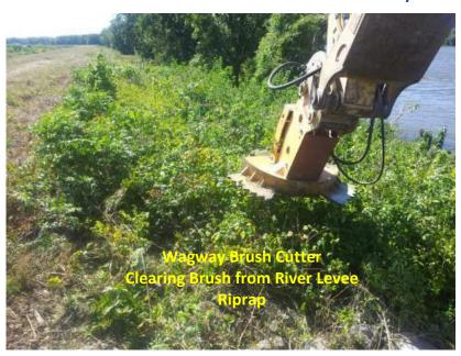
the removal of brush from ditch banks. Some time ago, the District added to its brush control capabilities purchasing a hydraulic thumb attachment as well as a used brush Wagway attachment for the Cat 324DL excavator. In particular, the thumb attachment on the 324 allows for the removal of brush by pulling it up off the ditch banks rather than having to dig it out. Removal of the brush with the thumb makes for a much cleaner approach and also allows the brush to
