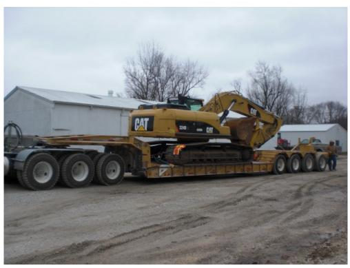
widen deck to nearly 12', which necessary for transporting our **largest** excavator. The four axle trailer and four axle tractor are also required for the District to haul equipment as heavy as 60 tons, the approximate weight of the Sny's Cat 350L reach long excavator. In the
